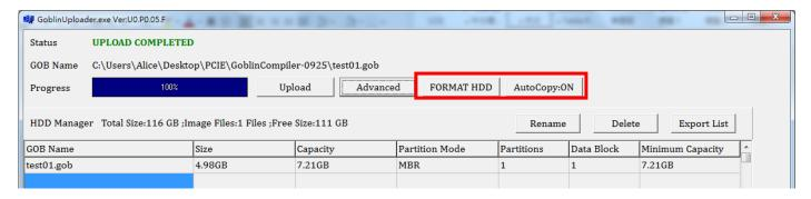
■ Format HDD: Format the internal SSD in the PCIE duplicator.
